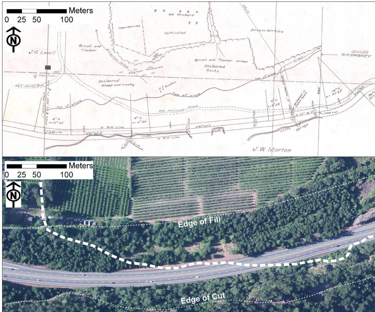
Figure 17. Top image shows a 1922 map of the recently completed HCRH highway, showing the position of the “Old Military Road;” bottom image shows the approximate alignment within the modern interstate highway prism, and the Wagon Road diversion from the modern corridor at about wagon road milepoint 24.6.
