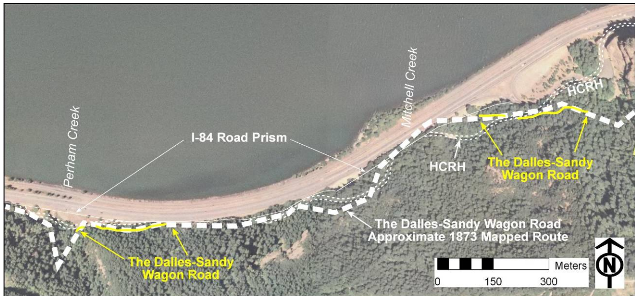
The corridor from the Mitchell Point Overlook to Perham Creek, showing the approximate 1873 mapped corridor, wagon road segments identified in the field, and the positions of the later HCRH and I-84 corridors.
