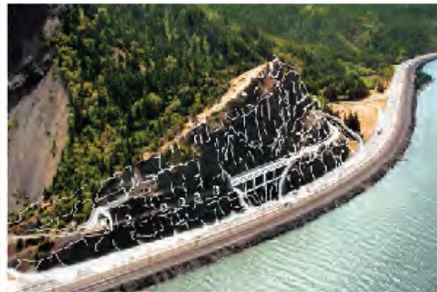
The Mitchell Point Tunnel Project would build a new tunnel through Mitchell Point and reconnect the two old highway sections at nearly the same grade as the old highway. The sketch overlaid on this aerial approximates the location of the old tunnel.
