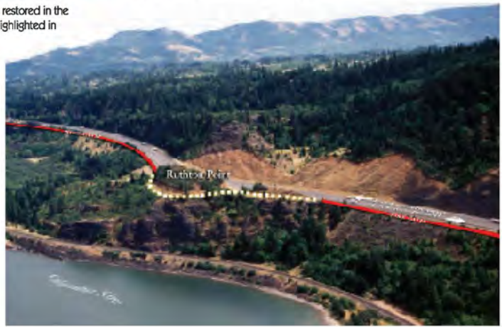
This aerial view of Mitchell Point approximates the location of the east portal and possible side adits or openings in the walls off the tunnel to the outside face of the cliff that would be akin to the original "Tunnel of Many Vistas".
